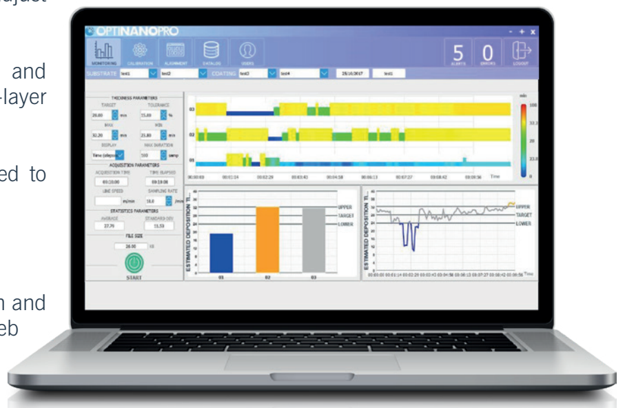
Software showing the variation of the monitored values across a set of 4 optical probes vs. set tolerance along the web while the coating is applied
